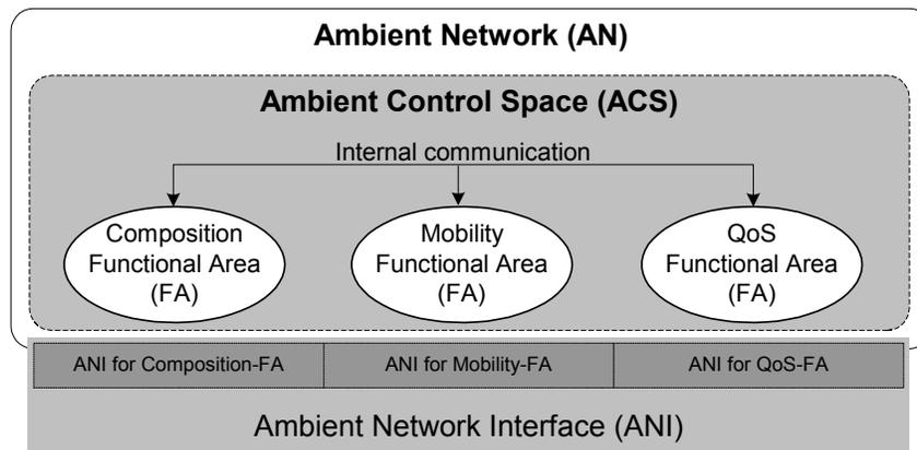
**Fig. 1: An example of the Ambient Network Architecture**
